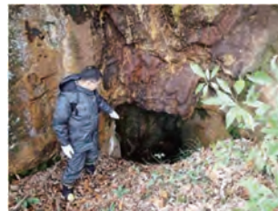
Contact of rainwater seeping underground with ore may generate acid water containing heavy metals. Therefore, it is necessary to monitor water from surrounding springs even at suspended and closed mines continually.
