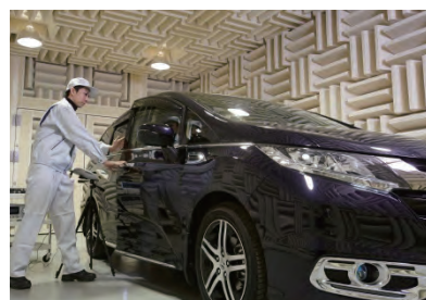
Testing using psychoacoustic technology to monitor the closing sound of car doors in an anechoic room (Mitsui Kinzoku ACT)
