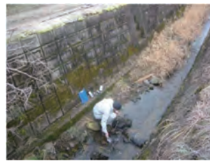
Contact of rainwater seeping underground with ore may generate acid water containing heavy metals. Therefore, it is necessary to monitor water from surrounding springs even at suspended and closed mines continually.
